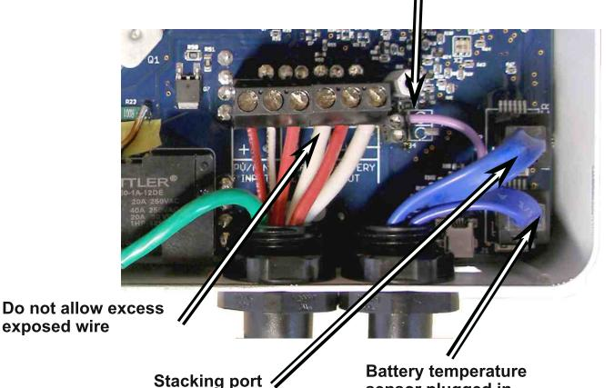
**Sample wiring** showing PV, Load, Battery, Whizbang Jr., BTS and stacking cable. Wires may exit through either conduit fitting.
