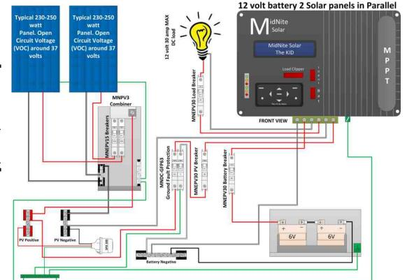
Both the input and output negatives must be connected to their own separate terminals readings and possible damage to the unit. Tying them together will cause inaccurate current
