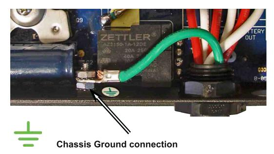
The screw, nut and terminal for grounding the chassis are included on all models. The chassis ground (equipment ground) is required in an NEC compliant system. The chassis of the KID is isolated from all internal KID circuitry.
