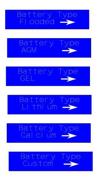
Stop on the correct battery type and then hit the right arrow key. It then takes you to the absorb voltage screen.
