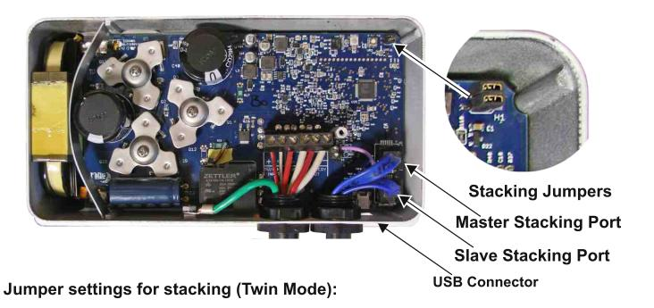
In the upper right corner of the circuit board there are two positions for placing jumpers. If not stacking (only one Kid) or stacking two Kids leave the jumpers off. The jumpers may be placed on one pin to be saved for later use. When stacking 3 or more Kids in "Follow Me" mode jumpers should be placed in both positions on the second and subsequent Kids. The jumpers should be oriented side to side (horizontally).
